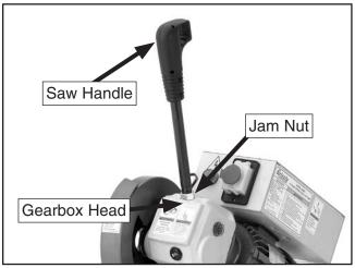
Figure 1. Attaching the handle.
